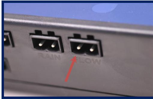
4. **Setup Parameters:** Refer to the manual to enable the flow sensor through the Cyber-Rain software. You will have to also choose what type of flow sensor is installed, DI or meter type.
